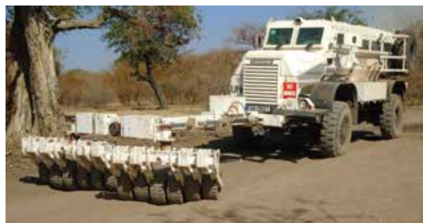
Route Verification carried out by TDI IRACT team along the suspected locations in Safahah area, CASSPIR MPV (Mine protected Vehicle) with Advance Roller System
